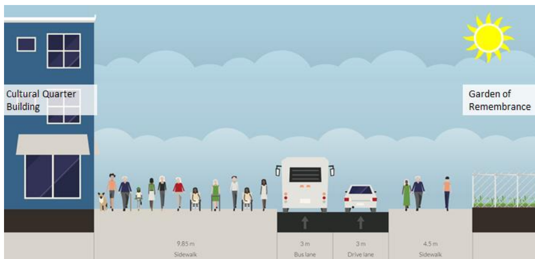
Figure 3.2: Option 2A: – Two 3m-wide traffic lanes, One lane for Public Transport and one for all traffic
